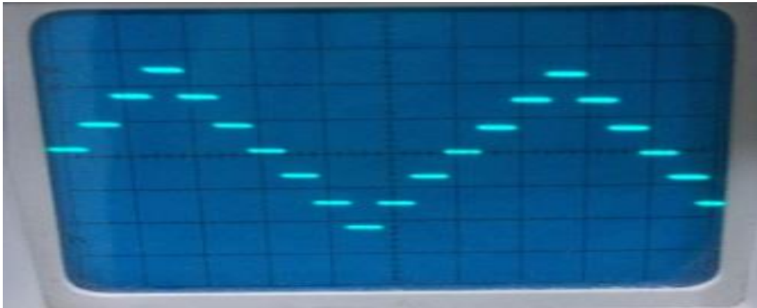
Fig.13 7 level multi- inverter waveform
